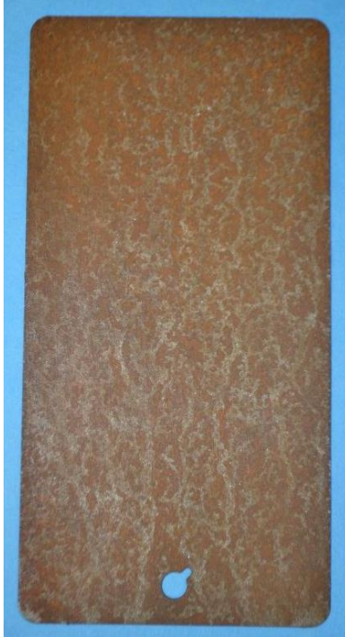
Figure 1: Rusty Steel (Wire Brushed)
